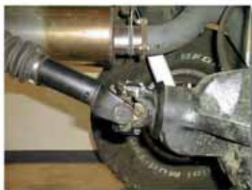
Rear (too low). Will not raise enough for C.V.!
