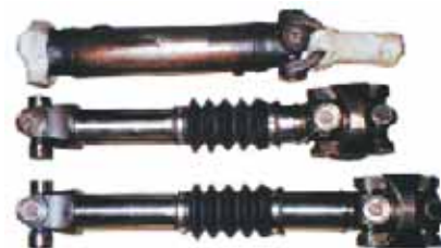
Stock driveshaft (top) vs. New fixed yoke driveshafts
