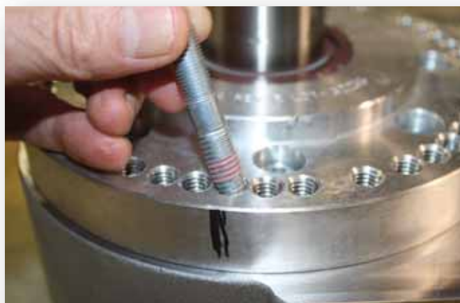
Rotation pattern located from the mark made on the outside of the Atlas index ring
