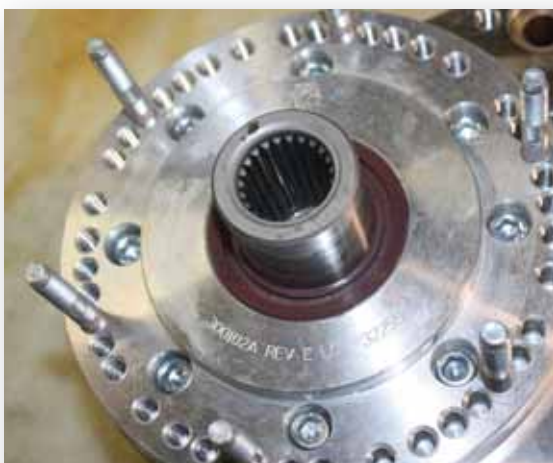
Install the stud bolts in same location all the way around the index ring
