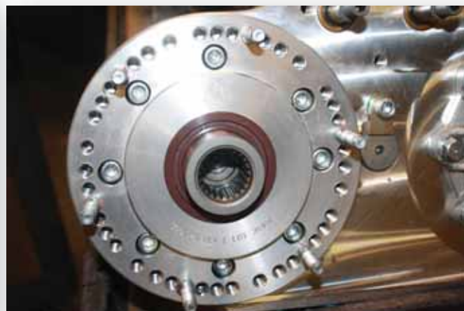
Stud bolts installed for a Jeep JK with the stock rotation
